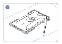
After turning the stand neck of the display counterclockwise for 10°, lift the stand neck to detach it from the device.
