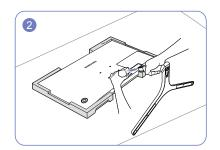
To disassemble the stand from the monitor, make sure to press the lower part of the monitor with one hand, and pull and sway sideways the stand with the other hand, as shown in the picture.
