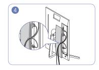
Arrange the cables against the bend tendency of the cables and pull the cables out of the COVER-REAR SUB grooves.
