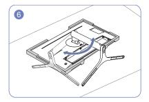
Turn the stand neck of the display clockwise for 90° to ensure that the stand neck of the display is put into place.
