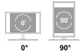
The on-screen display (OSD) menu items will automatically rotate when the screen rotates.
