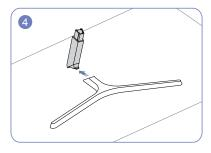
Remove the stand neck from the stand base by pulling it in the direction of the arrow as shown in the figure.
