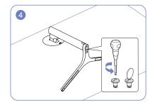
Turn the connecting screw at the bottom of the stand base to separate it.
